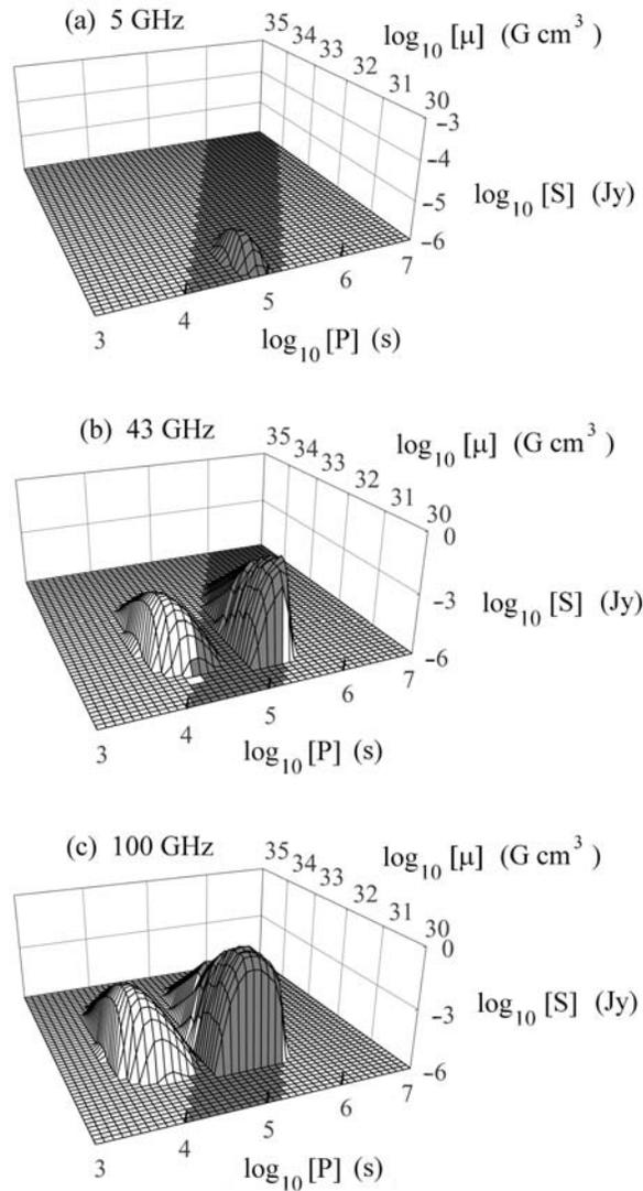
**Fig. 9** Flux density of loss-cone electron-cyclotron masers at 5, 43 and 100 GHz from a UI white-dwarf planetary system. The magnetic moment of the magnetic white dwarf  $\mu = 10^{30} \text{ G cm}^3$ , the number density of the loss-cone electron population is  $10^7 \text{ cm}^{-3}$ , and the mean energy of the electrons is 1 keV. The distance to the source is 100 pc. The gray band denotes the region in parameter space where detection is expected for the current instrumentation.
