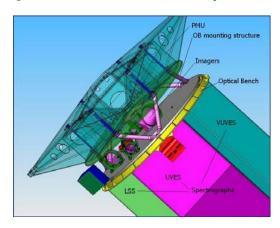
Fig.2 Instrumental Compartment, showing the location of the focal plane instruments.
