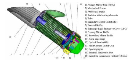
Fig. 1 General view of the T–170M telescope.
