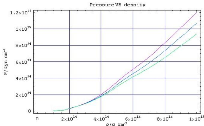
**Fig. 2** EOS for RMF210, RMF240 and RMF300, from the bottom up. The behavior of TNI2u, TNI6u and TNI3u is similar.
