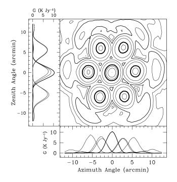
**Fig. 1** Contours of the ALFA telescope gain. Levels are at -1, -2, -3, -6, -9, -12, -15 and -19 dB from the central peak. The equivalent circular beam width (FWHM), averaged over all beams, is 3.35 arcmin at 1.42 GHz. The on-axis gain is approximately 10.4 K Jy<sup>-1</sup> for the central beam and  $\sim 8.2$  K Jy<sup>-1</sup> for the other six beams. The system temperature looking out of the Galactic plane is  $\sim 24$  K. (Paper I; Heiles 2004).
