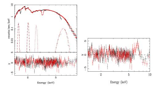
**Fig. 2 Left:** Top panel: HEG fi rst order spectra of 4U 1705–44 together with the best-fi t model (see Table 2). The discrete features included in the best-fi t model and described by Gaussians are also shown. Bottom panel: Residuals in units of  $\sigma$  with respect to the best fi t model. **Right:** Residuals in units of  $\sigma$  with respect to the simple Comptonization continuum when the iron line and other low energy Gaussians are not included in the model.
