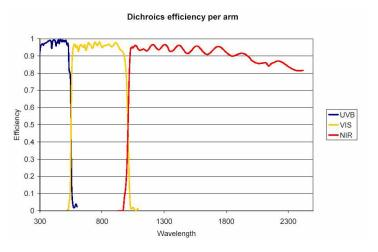
Fig. 3 Efficiency of the X-shooter dichroics.
