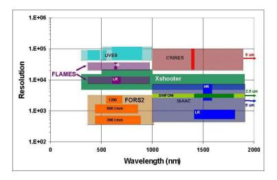
**Fig. 1** Properties of VLT spectrographs in the resolving power versus wavelength plane U to H range). Note that by the time X-shooter will be in operation the FORSes and ISAAC will be beyond their guaranteed lifetime.
