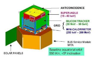
Fig. 1 The AGILE instrument is light (total payload weight of  $\sim 130$  kg) with a size of  $\sim 63 \times 63 \times 58$  cm<sup>3</sup>.
