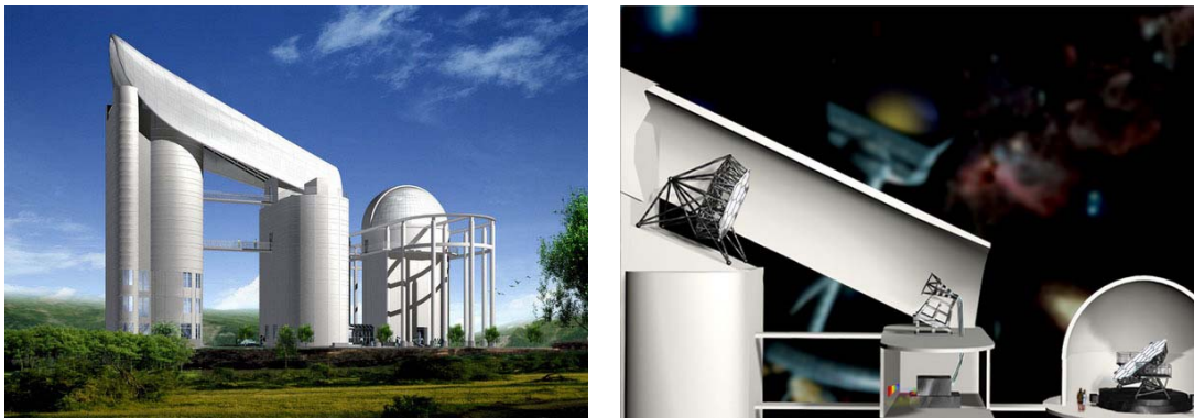
Fig. 1 LAMOST model. Left: exterior view; Right: optical part with encloser.
