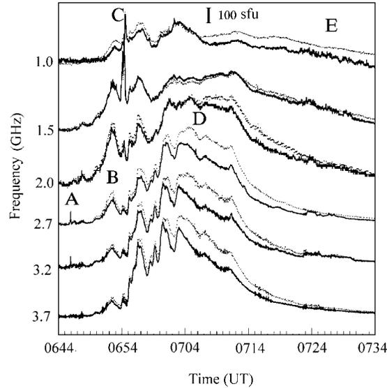
Fig. 1 Spectrogram (time profiles) of radio bursts of 1998 September 23 at selected frequencies, thin lines for left polarization, thick lines for right polarization. Capital letters A, B, C, D and E mark the places of the four groups of Type III bursts and the period of the Type I-like noise storm, respectively.
