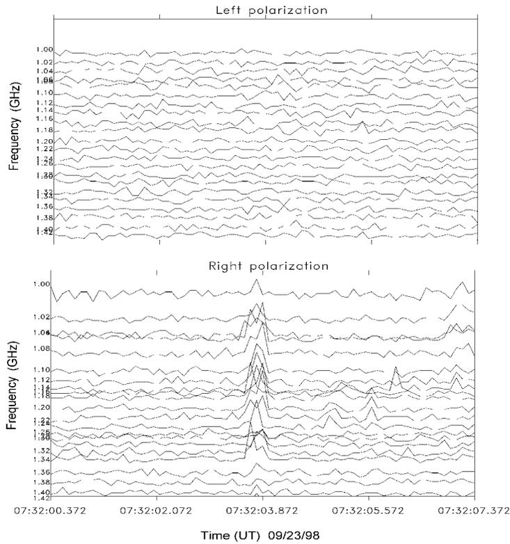
Fig. 5 Enlarged fast fine structures of one Type III burst with positive frequency drifting rate associated with the Type I-like noise storm.
