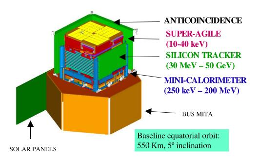
Fig. 1 The AGILE instrument size is  $\sim 63 \times 63 \times 58.5$  cm<sup>3</sup> for a total payload weight of  $\sim 130$  kg.
