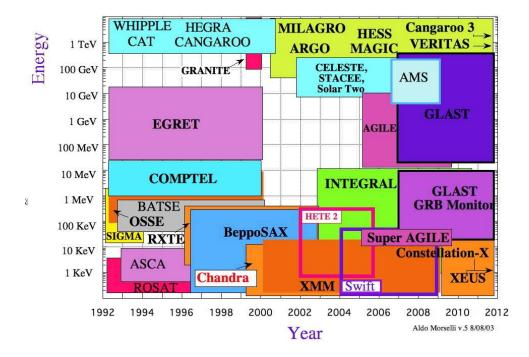
**Fig.7** Timeline schedule versus the energy range covered by present and future detectors in X and gamma-ray astrophysics.
