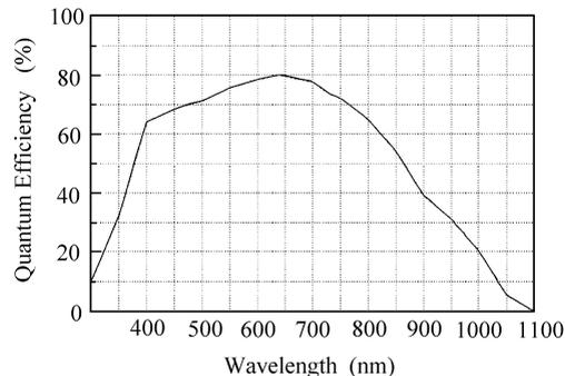
Fig. 2 Quantum efficiency of NAOCES TEK CCD as function of wavelength.
