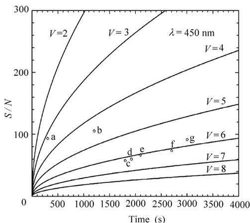
Fig. 3 Expected  $S/N$  at 450 nm as a function of exposure time for stars of different magnitudes. Circles represent the observational data. The name and visual magnitude of the labelled stars are: a— HD155763,  $m_v = 3.17$ ; b— HD144206,  $m_v = 4.71$ ; c— HD71148,  $m_v = 6.32$ ; d— HD127334,  $m_v = 6.38$ ; e— HD110897,  $m_v = 6.00$ ; f— HD71148,  $m_v = 6.32$ ; g— HD99747,  $m_v = 5.80$ .
