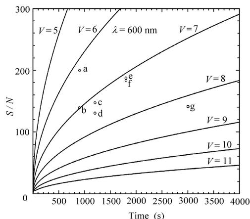
Fig. 4 Expected  $S/N$  at 600 nm as a function of exposure time for stars with different magnitudes. Circles represents the observational data. The labelled stars are: a— HD7351,  $m_v = 6.33$ ; b— HD223617,  $m_v = 6.96$ ; c— HD178717,  $m_v = 7.18$ ; d— HD170970,  $m_v = 7.42$ ; e— HD178717,  $m_v = 7.18$ ; f— HD200063,  $m_v = 7.28$ ; g— HD22694,  $m_v = 8.24$ .
