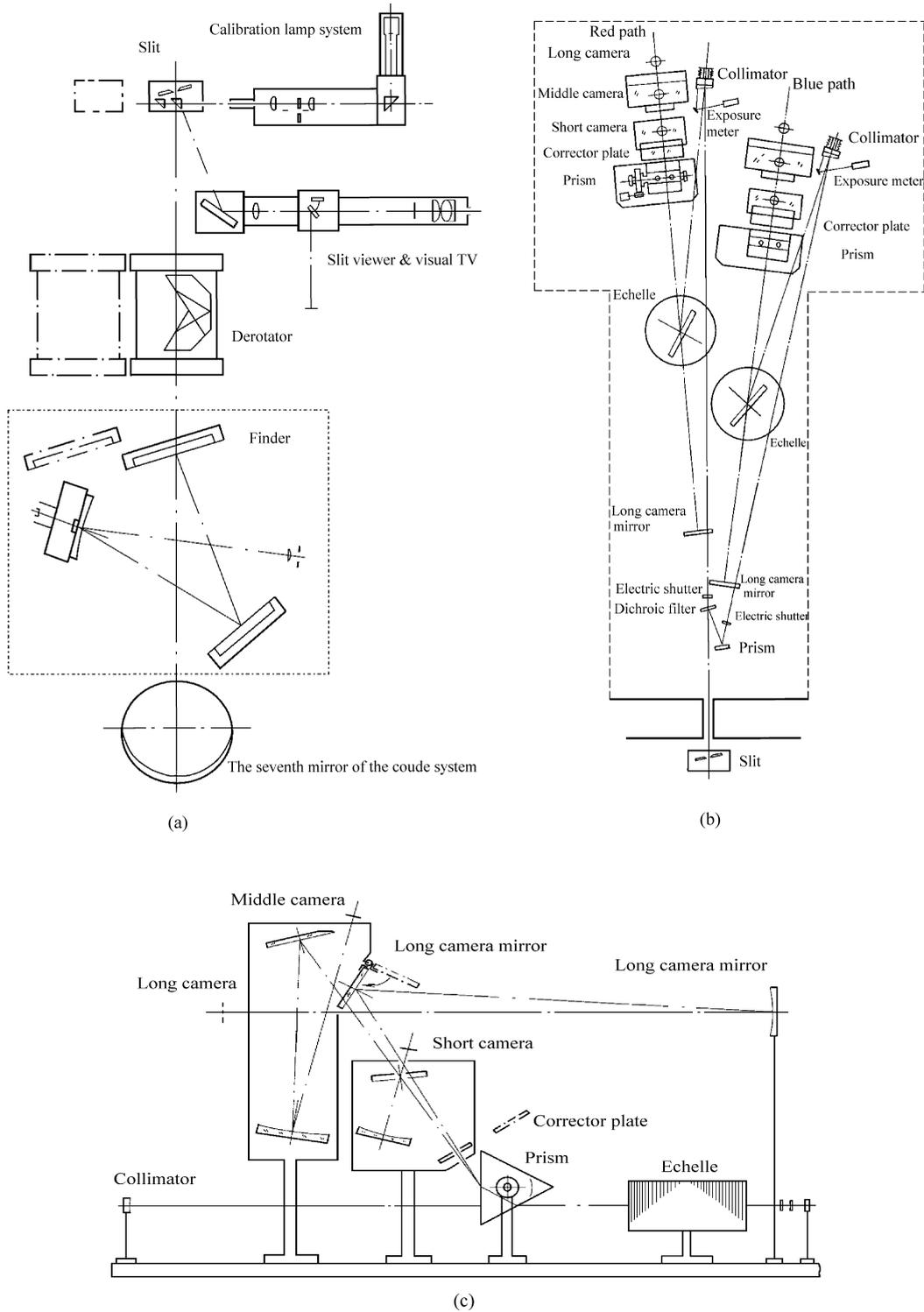
Fig. 1 Optical layout of the NAO coudé echelle spectrograph (a) top view of NAOCES optical layout before slit; (b) top view of NAOCES optical layout after slit; (c) side view of NAOCES optical layout after slit.
